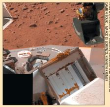
Scoop on robotic arm hangs above TEGA after dropping another load of soil into the instrument. Red soil covers door area.
